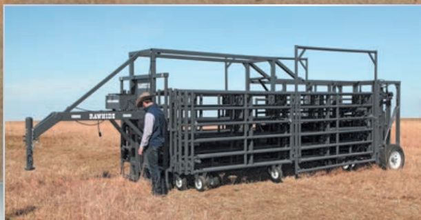
Once unhooked from truck, set corral main frame down on the ground.
