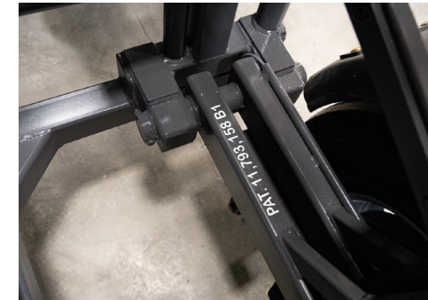
Patented torsion axle suspension U.S. Patent No. 11,793,158
